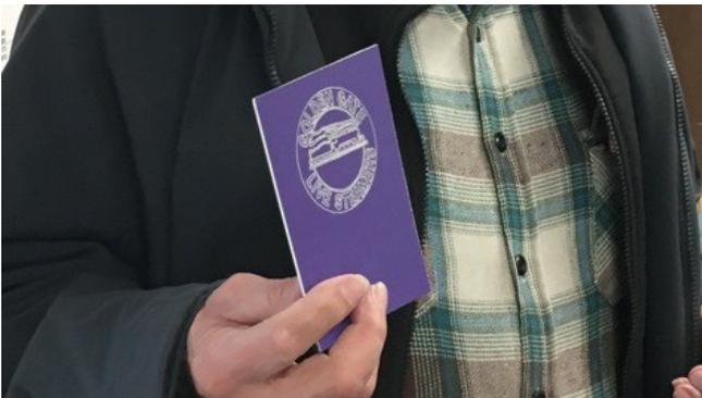
Jerry Kimberlin decided to have a go at making a GGLS members badge out of some 1/16” thick plastic sheet. First, he scanned an existing badge as he didn't have access to the original artwork, converted the image to a Bit map using Photoshop, then F-Engrave to generate G-code (Geometric CODE) which is
