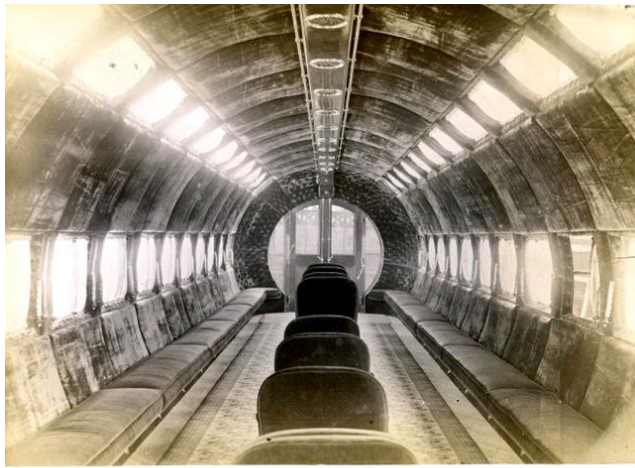
MEIGS RAILWAY—Interior of Car No. 1, "EGENIA BEATRICE"—72 seats—Weight of Car, 34,000 lbs. Length, 51 ft. 2 in. Fireproof Circular Car. June 1, 1886.
