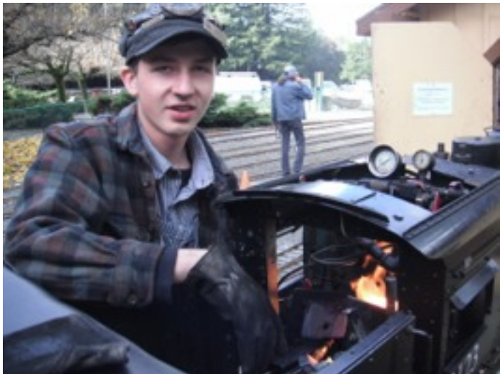
David Waterman testing the newly installed double jet oil burner in the Johnson Pacific.
