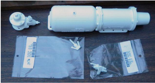
Rich brought along one of the truck sets with the fabricated body bolster (very nice) and 3D printed brake cylinder and valve parts made by Shapeways.
